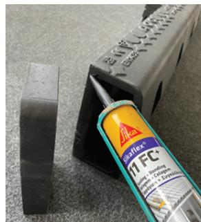
**3** Once cut, install the end cap using a recommended sealant such as Sikaflex 11FC or Geocel 945.
